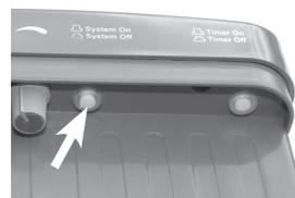
**2. Position OFF :** The pump is switched-off. The accumulator is charged via the solar module and the electric energy is stored. The LED „System“ is not illuminated.
